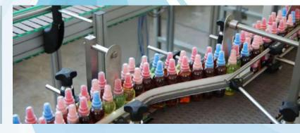
The Pick & Place systems are compact and versatile solutions for the handling of several products; they are used to create multi-layer configurations, for the handling/transfer or inserting products into trays, boxes, blister packs, etc. Each pick and place is customized for the product to be treated and for the required application, ensuring the necessary flexibility for every application.
