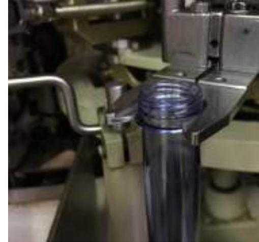
Pliers and clamping preform details heated by blowing station
