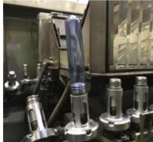
Replacing heating oven details necessary to changing diameter or height of the neck finish
